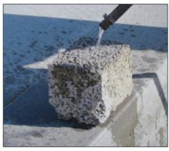
Pervious concrete is made without sand so that water can pass through its pores.
